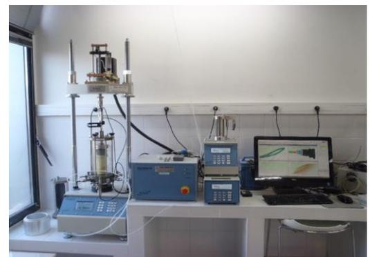
Triaxial cyclic test machine (Sémofi)
