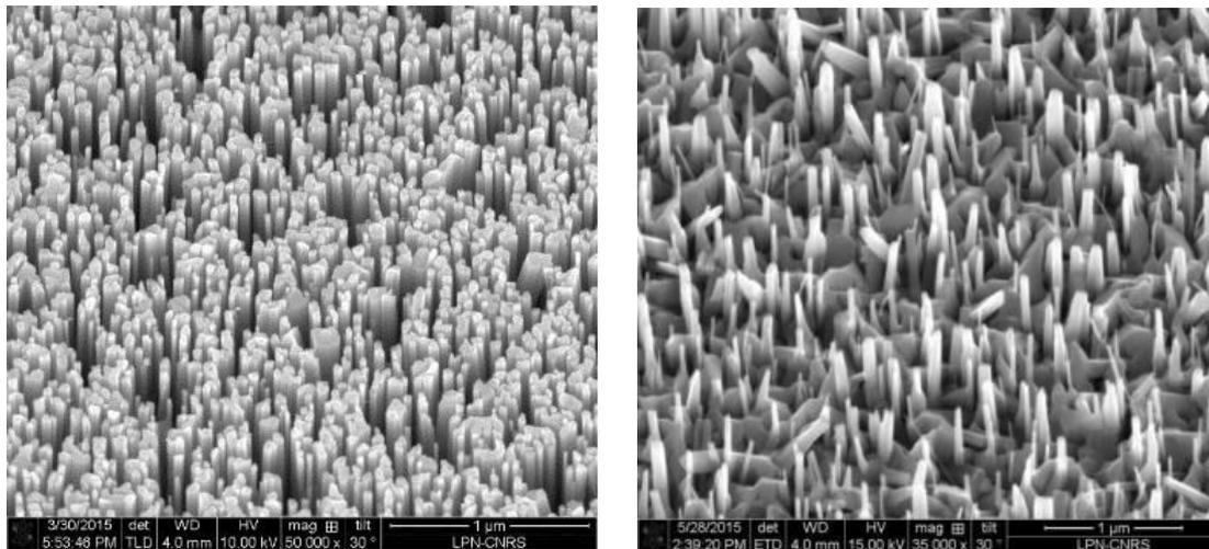
Fig. 1. Images obtained by scanning electron microscope of two samples of different morphology (dense nanowires on the left, thin nanowires on the right)
